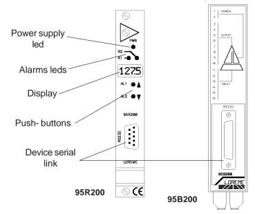
The 95B200 front panel is composed of a SUB - D 25 pins connector. The device configuration is make will be making by this RS 232 link .
