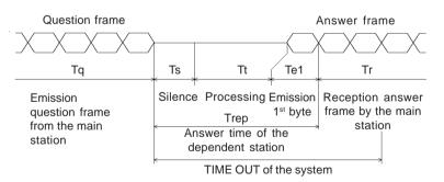
The time beyond which the device does not answer is called "**TIME OUT**". It depends on the transmission parameters (speed, format) and the type of the function asked (reading, writing). This time must be defined by the user and must be superior to the answer time of the device.
